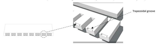
$\frak{X}$ Tinned trapezoidal grooves on the tips of Gate and Source
